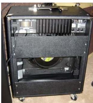
The rear panel boasts some great features as well. A 1/4" TUNER out, a balanced XLR out, a GROUND LIFT switch that disconnects the LINE OUT ground
