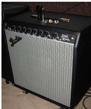
LEVEL and the MID FREQUENCY. The MID LEVEL adjusts the tone at the frequency set by the MID FREQUENCY. This allows a great deal of latitude in mid-range tone coloration. And there is a BASS control for low frequency tone adjustment.
